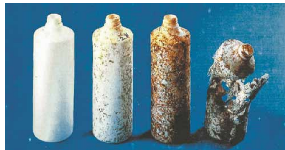
An eco-friendly, biodegradable polyactic acid, which is decomposed by microorganisms found in soil, is under development by Japanese researchers. The bottles pictured represent various stages of the plant-based plastic's decomposition. From left — zero weeks, two weeks, four weeks and six weeks. JAPAN BIOPLASTICS ASSOCIATION
